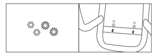
Install tail light to rear rack with these 2 sets of nuts and washers.
