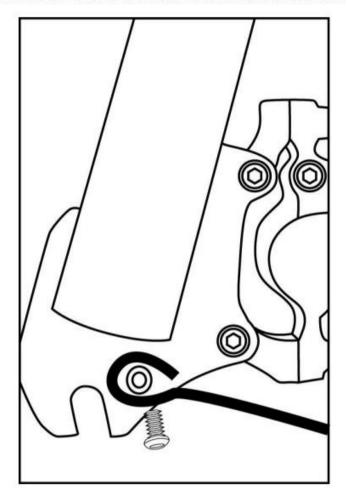
5, Mount rear fender by fixing the spokes to frame first, with 1x allen bolt on each side
