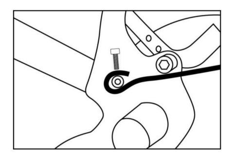
5.2 Mount allen bolts and washers to place (1) and (2). Press tires to access narrow position.
